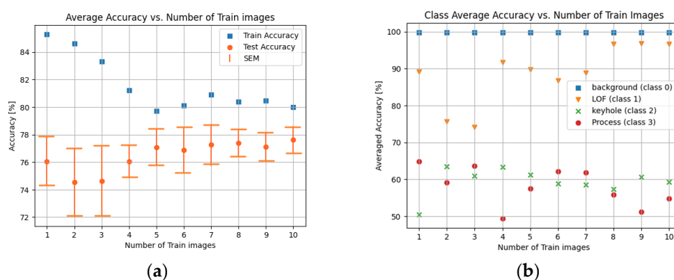
Figure 5. (a) Overall averaged accuracy of RF classifier vs. increasing number of training images, (b) each class averaged accuracy of RF classifier vs. increasing number of train images.
