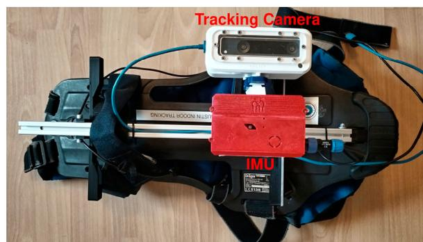
**Figure 2.** Sensor assembly mounted on the firefighter equipment.
