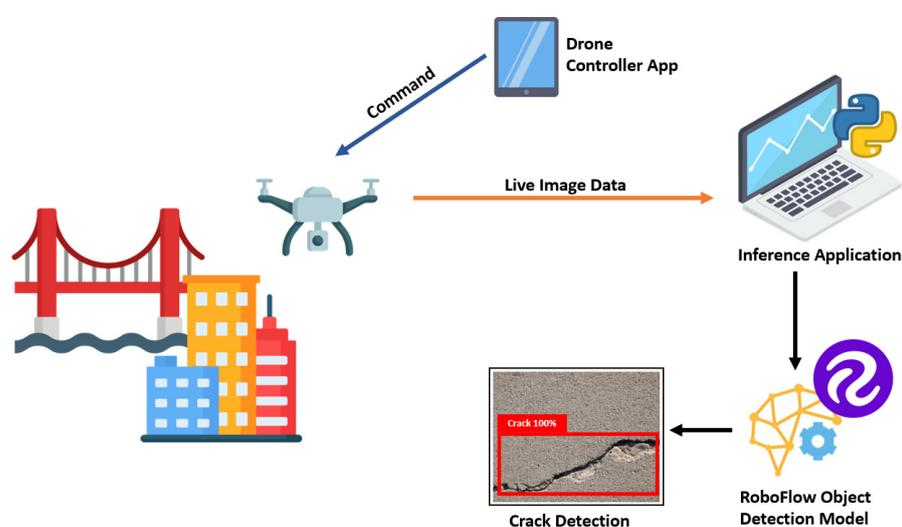
Figure 1. System Architecture.
