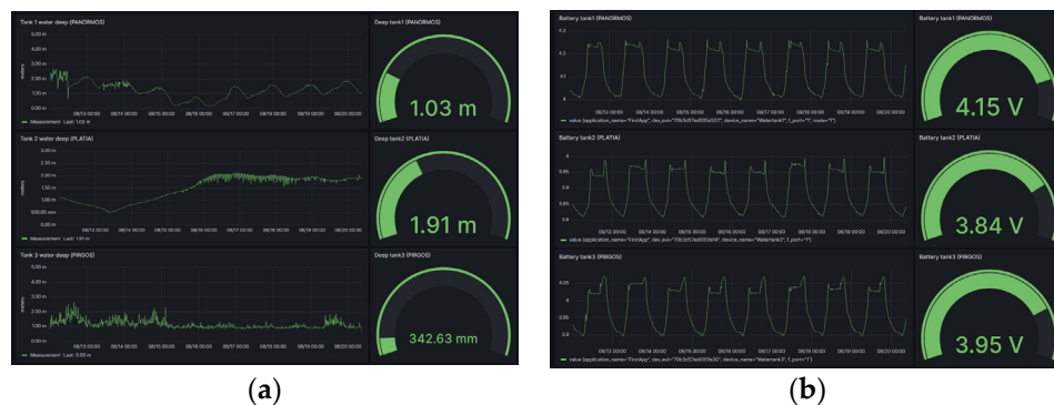
Figure 6. Grafana lab visualization interface. (a) Water tanks depth. (b) Battery voltage.
