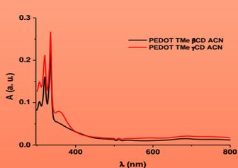
Figure 2. Electronic absorption spectra in ACN
