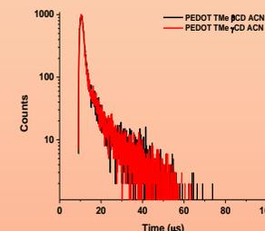
Figure 5. Phosphorescence lifetime in ACN with  $\lambda_{ex}=355$  nm
