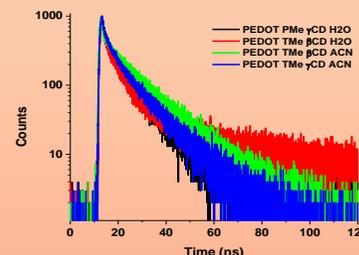
Figure 4. Decays in  $H_2O$  and ACN with  $\lambda_{ex}=375$  nm
