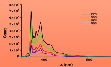
Figure 3. Fluorescence spectra of PEDOT TMe  $\beta$ CD in ACN
