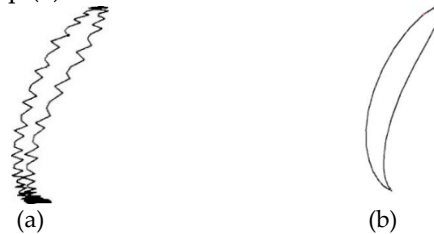
Figure 5. (a) Impedance plane plot when spectral leakage occurs, (b) Normal impedance plane.
