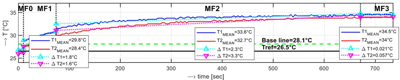
**Figure 4.** Concatenated sequences from thermo-sensors MCP1, MCP2 together with fitted linear regressions, calculated mean and  $\Delta T$  values; concatenate for measuring phases MF0-3,  $T_{REF} = 26.5^\circ\text{C}$ , baseline for MF1-3 measurements is  $28.1^\circ\text{C}$ ,  $t_{DUR}=738$  s, person P1M.
