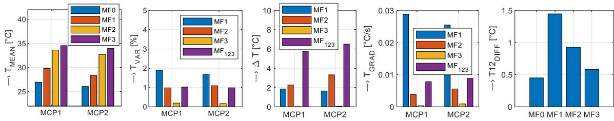
**Figure 5.** Statistical parameters determined from temperature sequences T1, T2 from thermo-sensors MCP1, MCP2 introduced in Figure 4 (from left to right): mean values, relative variations,  $\Delta T$  values, gradients, and differential T12 values between MCP1’s and MCP2’s for each of three measurement phases (MF1-3); final values MF123 determined for whole measurement.
