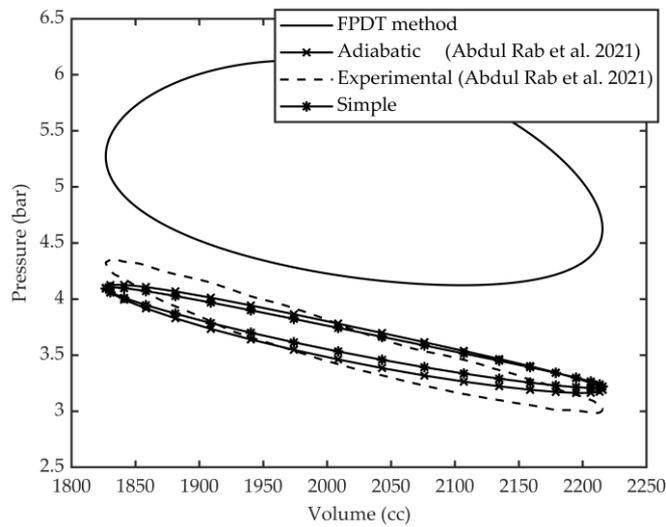
Figure 1. Comparison of FPDT model with other isothermal model and experimental data.
