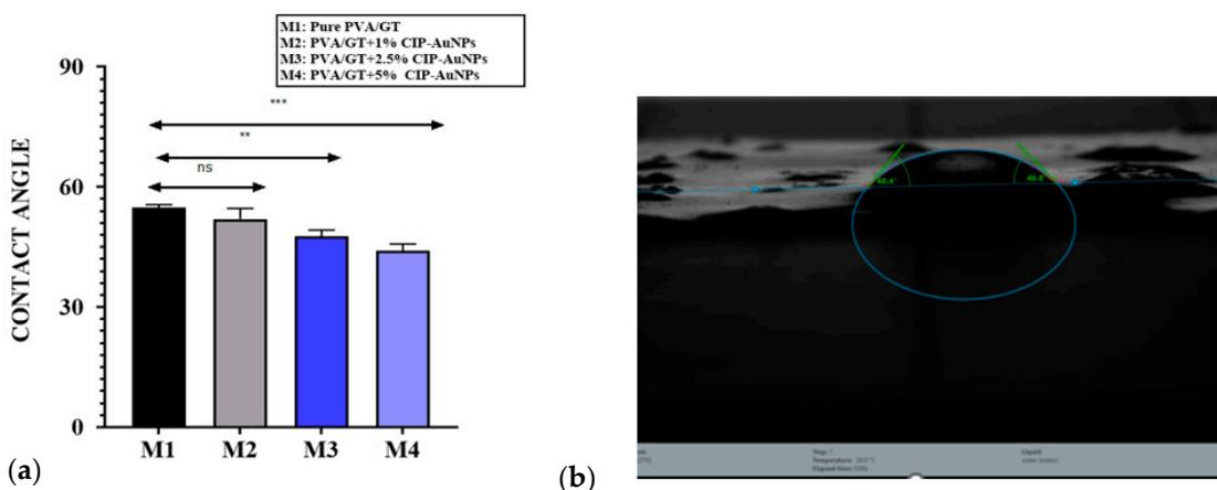
**Figure 3.** Contact angle of (a) Pure PVA/GT, PVA/GT loaded with 1% CIP-AuNPs, PVA/GT loaded with 2.5% CIP-AuNPs, and PVA/GT loaded with 5% CIP-AuNPs. ns shows statistically insignificant results as *p* value is greater than 0.005 while \*\*\* and \*\* shows statistically significant results as *p* value is less than 0.005. (b) Contact angle of PVA/GT loaded with 5% CIP-AuNPs.
