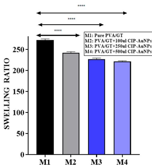
**Figure 2.** Swelling ratio of Pure PVA/GT, PVA/GT loaded with 1% CIP-AuNPs, PVA/GT loaded with 2.5% CIP-AuNPs, PVA/GT and PVA/GT loaded with 5% CIP-AuNPs. \*\*\*\* shows statistically significant results as *p* value is less than 0.005.
