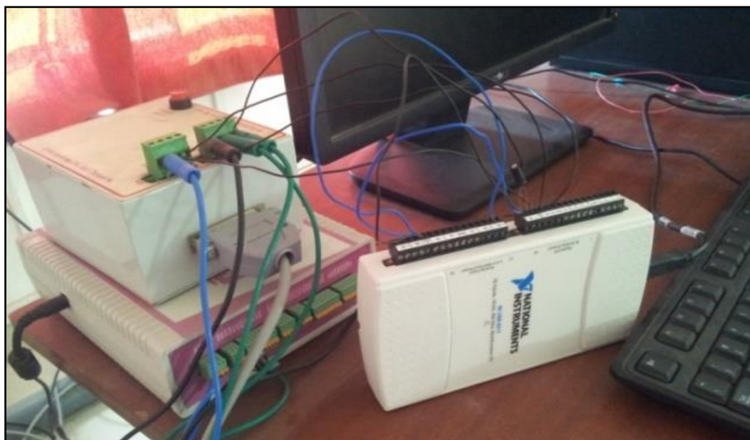
Figure 2. Interfacing computer using NI-DAQmx 6211 data card.
