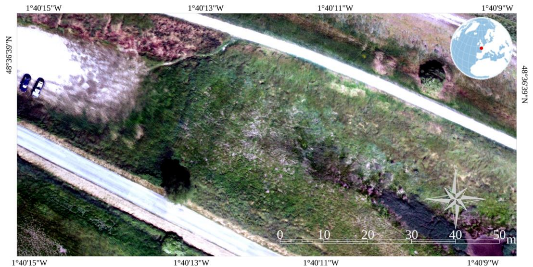
Figure 1. Blue-green-red composite imagery of the study site and its global location (11 385 × 5 538 pixels; 0.01 m pixel size; 23 626 927 points).
