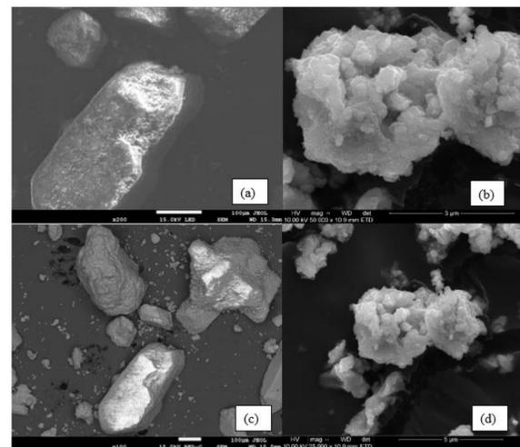
**Figure 1:** SEM images of NaHCO<sub>3</sub> sorbent - (a) and (c) and Ca(OH)<sub>2</sub> sorbent - (b) and (d)
