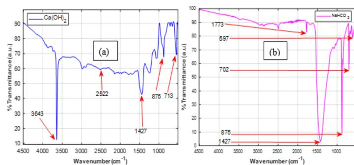
**Figure 3:** FTIR spectrum of (a) Ca(OH)<sub>2</sub> and (b) NaHCO<sub>3</sub> (nahcolite).
