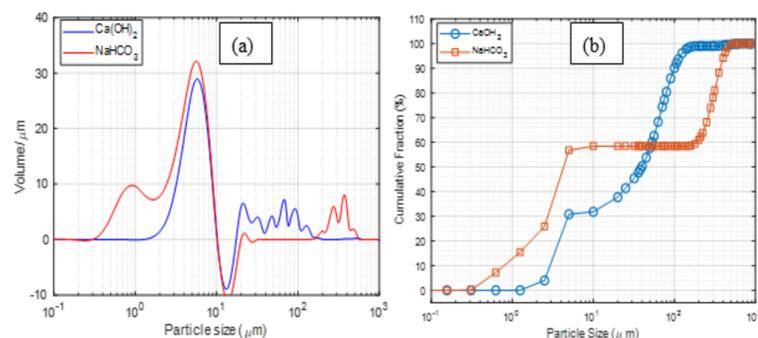
**Figure 2:** (a) Particle size distribution and (b) reagent cumulative distribution of the Ca(OH)<sub>2</sub> and NaHCO<sub>3</sub>
