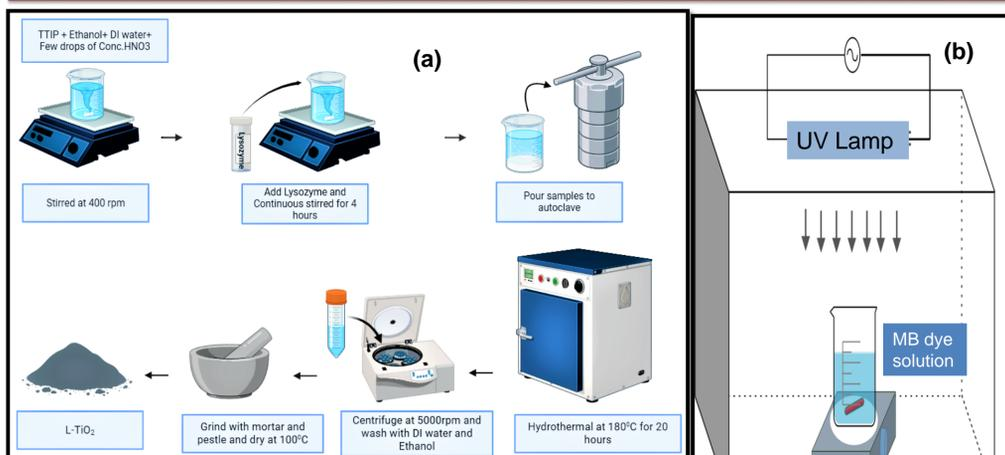
Fig 2 (a): Experimental diagram for synthesis of TiO<sub>2</sub>/L-TiO<sub>2</sub> (b) Photocatalytic Setup
