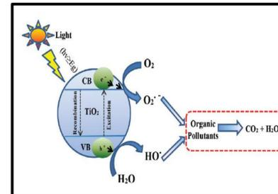
Fig 9: Mechanism of Photocatalytic degradation of dyes in UV light irradiation
