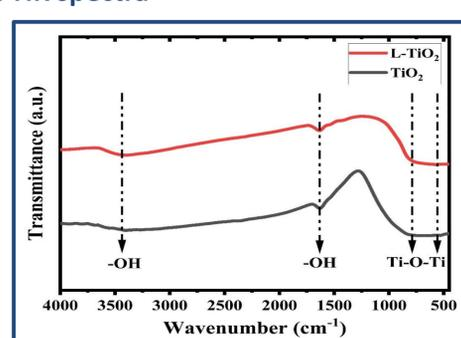
Fig 4: FTIR spectra of TiO<sub>2</sub>/L-TiO<sub>2</sub>
