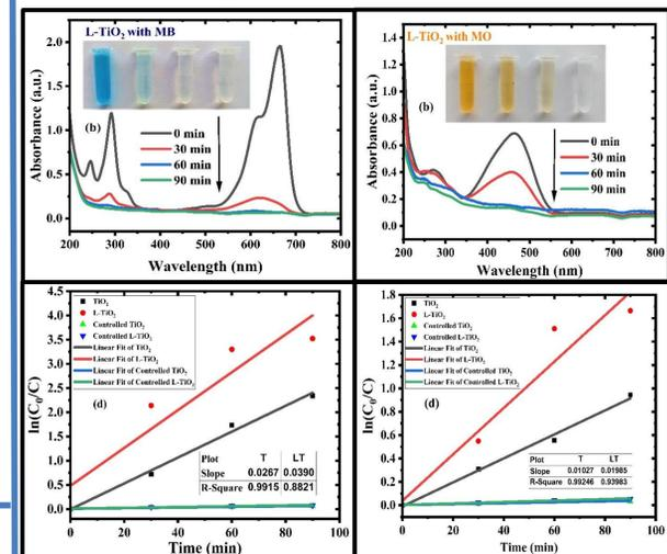
Fig 8: Degradation of MB and MO using L-TiO<sub>2</sub>
