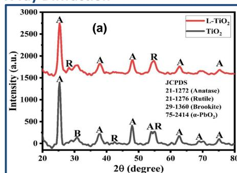
Fig 3 (a): Crystal structures of TiO<sub>2</sub>/L-TiO<sub>2</sub>
