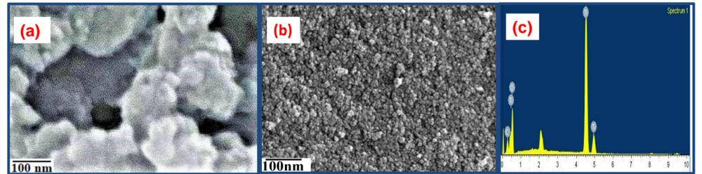
Fig 5: FE-SEM images of (a) TiO<sub>2</sub> (b) L-TiO<sub>2</sub> and EDS analysis of L-TiO<sub>2</sub>
