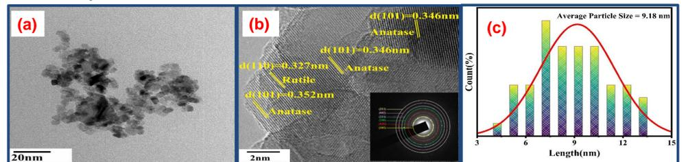
Fig 6: HR-TEM analysis of L-TiO<sub>2</sub> at (a) 20 nm (b) 2nm and (c) Histogram plot of L-TiO<sub>2</sub>
