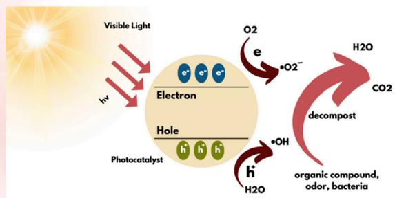
Figure 1. Photocatalytic Degradation Mechanism
