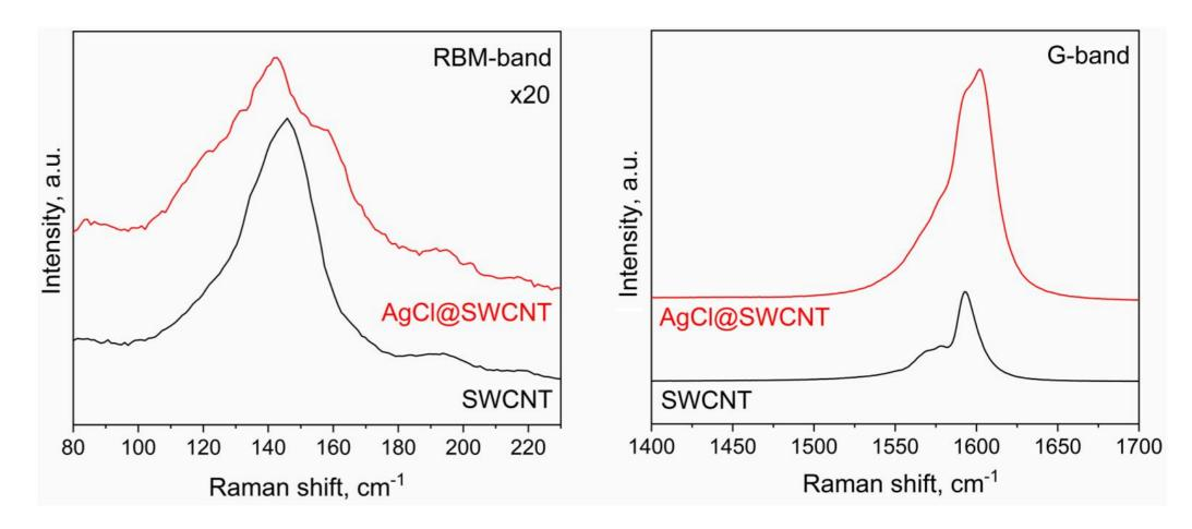
Moreover, the electronic properties of filled SWCNTs are modified.
