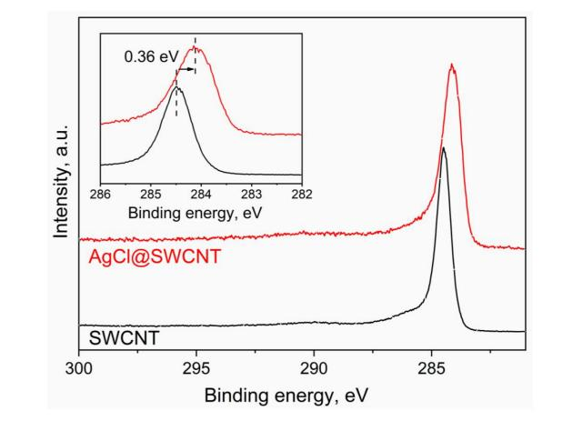
The C 1s X-ray photoelectron spectroscopy data of the silver chloride-filled SWCNTs [2]. Copyright 2023 by the authors. Licensee MDPI, Basel, Switzerland. This article is an open access article distributed under the terms and conditions of the Creative Commons Attribution (CC BY) license.
