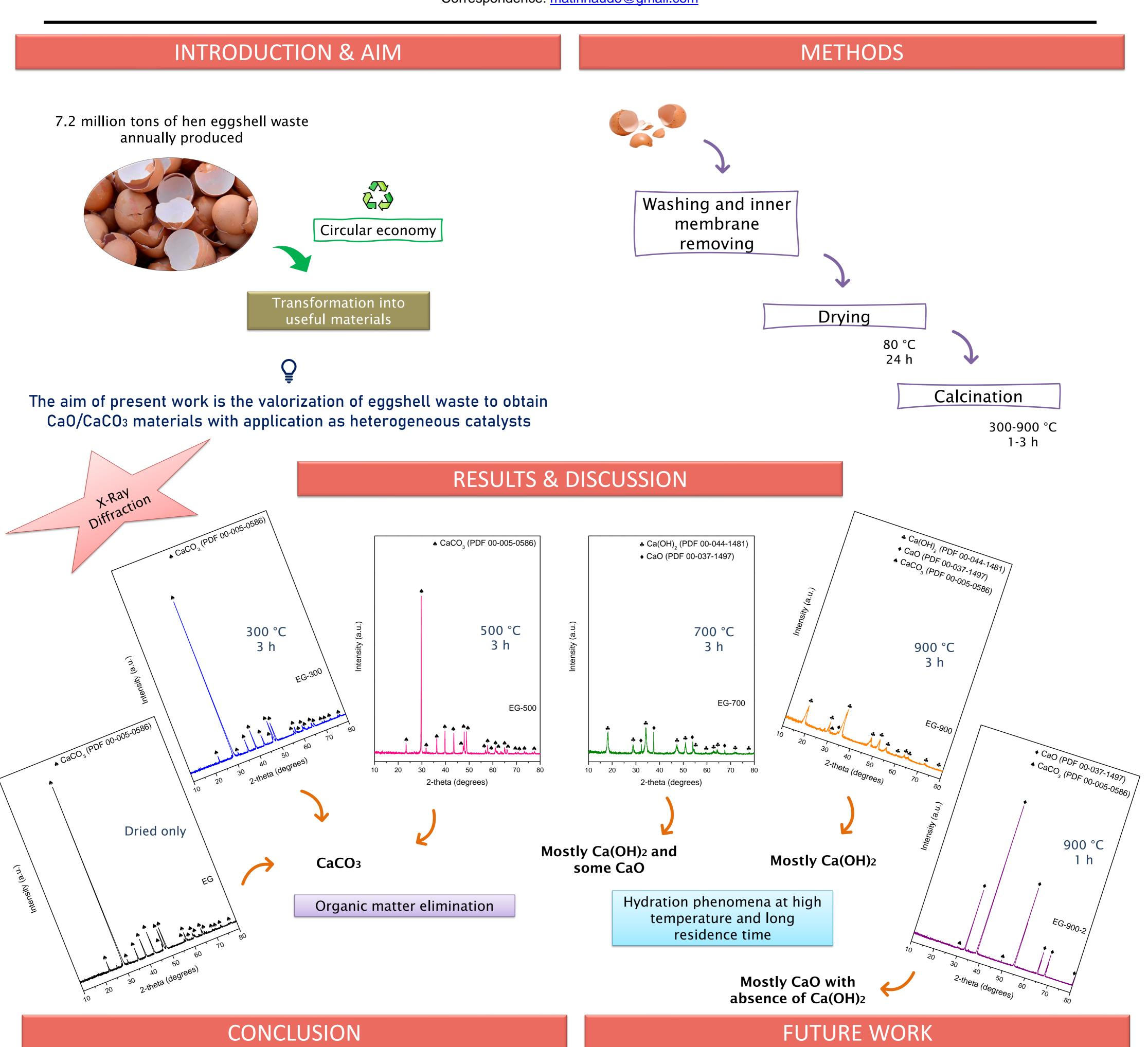
Physicochemical changes observed were correlated with the thermal treatments applied, evidencing the transformation from CaCO<sub>3</sub> to CaO and also the formation of Ca(OH)<sub>2</sub>. Considering this preliminary results, prepared solids could be useful as base catalysts in different heterogeneous reactions.
