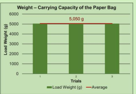
Figure 2. Weight-Carrying Capacity of the Handmade Paper Bag
