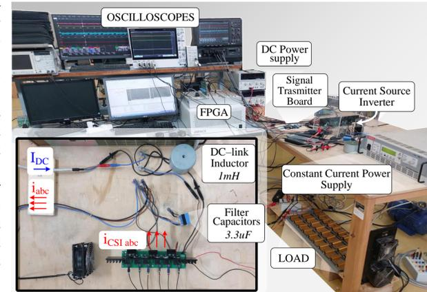
The purpose of this test is to display the experimental waveforms of the converter and verify the accuracy of the simulated system model.
