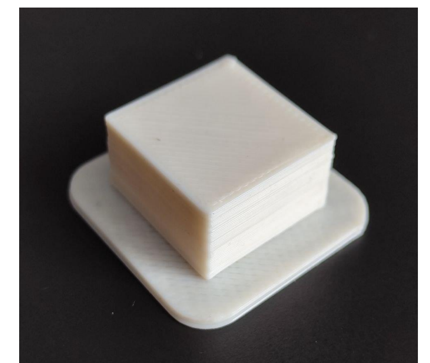
Photos of extruded filament and printed sample from CTS-b-PCL (1:2) composition
