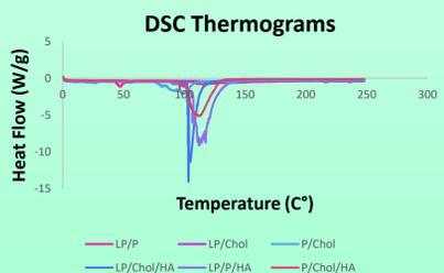
DSC thermograms of on phosphatidylcholine (LP), cholesterol (Chol), poloxamers (P) and hyaluronic acid (HA) and complexes used for nanoparticle preparation.
