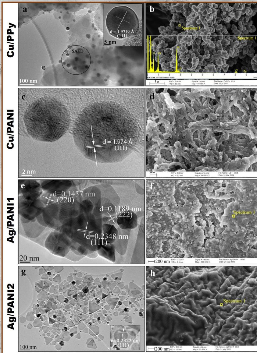
Fig. 1 TEM and FESEM images of MetNPs/polymer nanocomposites
