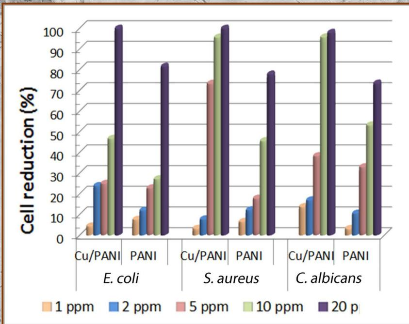
Fig. 2 Concentration-dependent reduction ability of the Cu-PANI and PANI on *E. coli*, *S. aureus* and *C. albicans*, over 1 h incubation time
