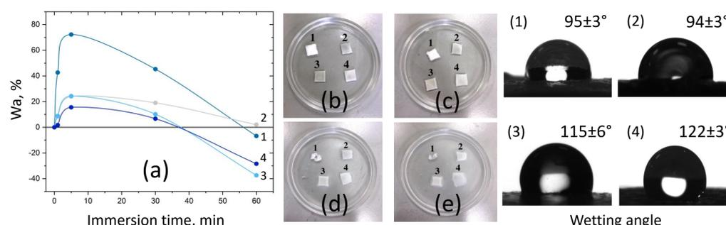
**Figure 2.** Kinetics of plate degradation in PBS (a) and corresponding images: at the initial moment of immersion (b); after 5 min in PBS (c); after 30 min in PBS (d); after 1 h in PBS (e); where 1 - Gel, 2 - Gel/HA; 3 - Gel/HA/Gla; 4 - Gel/HA/Gla+Ca<sup>2+</sup>
