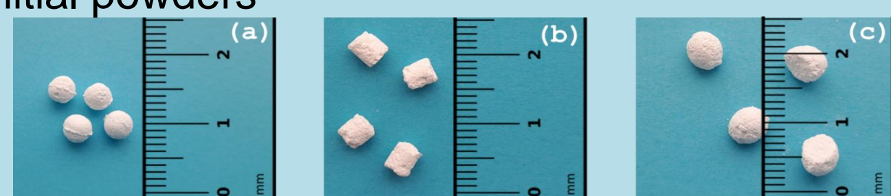
Figure 3. The shape of the granules: a – spheres, b – cylinders, c - hemispheres
