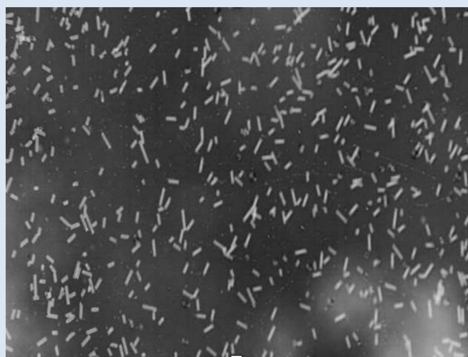
Figure 1: Optical polarizing photographs of silica and microrods (right) and Schematic diagram of a planar cell preparation (left).
