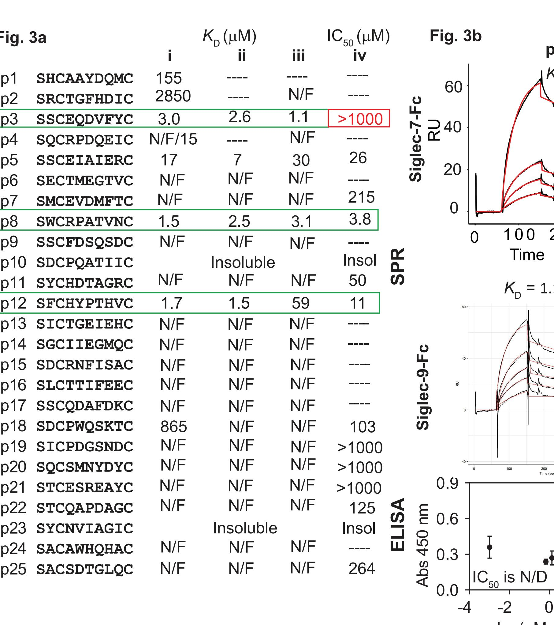
**Figure 3.** A) SPR evaluation of binding of 25 peptides to (i) Siglec-7-Fc; (ii) Siglec-7; (iii) Siglec-9 and (iv) inhibition of GD3:Siglec-7 interaction measured by ELISA. B) Surface plasmon resonance and ELISA binding traces of the three most active macrobicycles, p3, p8 and p12.
