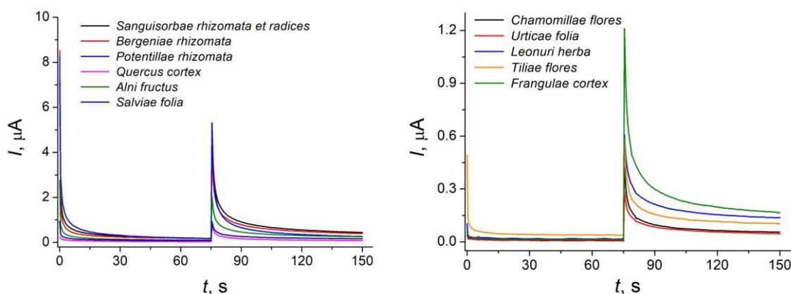
**Figure 2.** Two-step background subtracted chronoamperograms of 50 µL of medicinal plant extracts at the GCE modified with a mixture of 1 mg mL<sup>-1</sup> CeO<sub>2</sub> and SnO<sub>2</sub> NPs. Supporting electrolyte is phosphate buffer pH 7.0, E<sub>1</sub> = 400 mV, E<sub>2</sub> = 900 mV.
