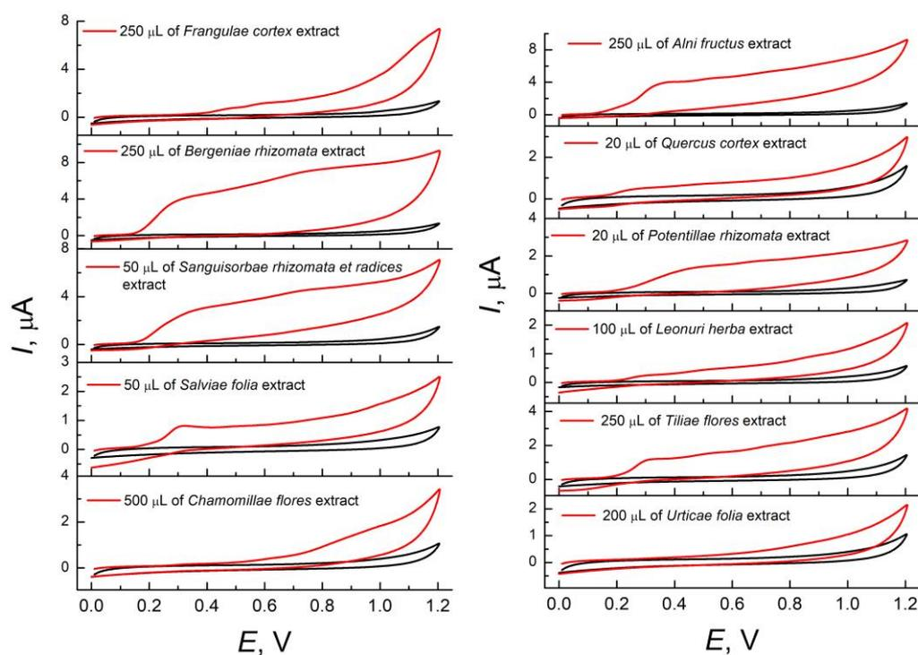
**Figure 1.** Cyclic voltammograms of medicinal plant water extracts on bare GCE in phosphate buffer pH 7.0. Potential scan rate is 100 mV s<sup>-1</sup>.
