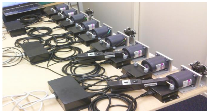
Figure 2. Multiple motor fault signature testbed.
