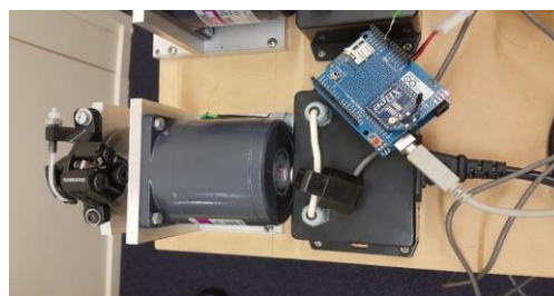
Figure 3. Arduino setup for wireless current monitoring.
