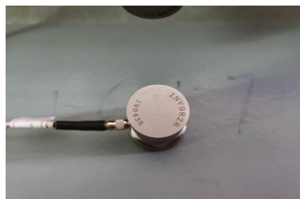
Figure 1. Adopted INV9828 ICP piezoelectric accelerometer.
