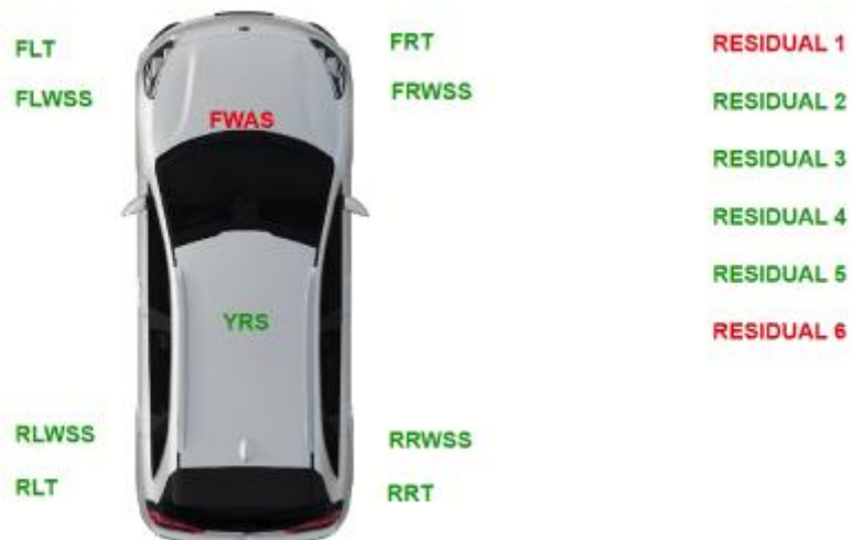
Figure 11. Steering Angle Fault on HMI Screen.
