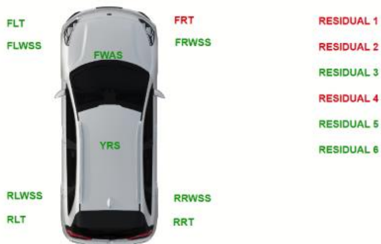
Figure 9. Right Front Tire Fault on HMI Screen.
