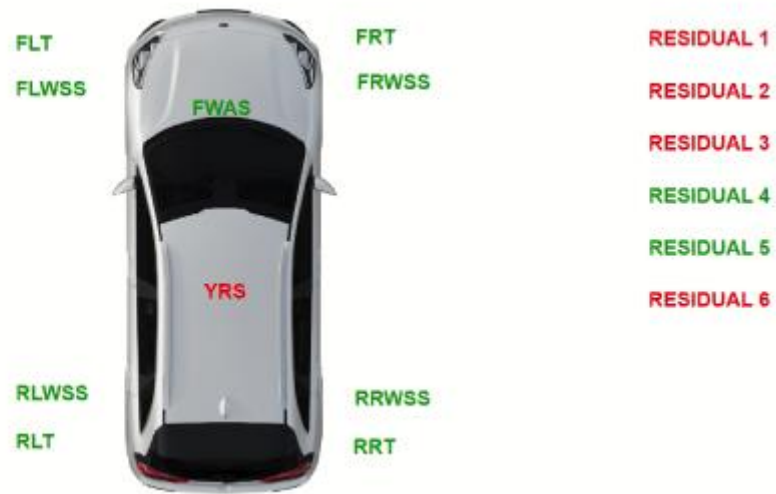
Figure 10. Yaw Rate Fault on HMI Screen.
