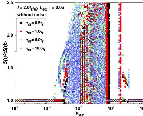
Under very weak OFB stationary solution bifurcates first into a stable limiting cycle characterizing PO. The HB point is moved to lower values of the OFB strength  $K_{ex}$  by increasing  $\tau_{nr}$ .
