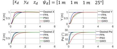
Based on the obtained results, the techniques provide an optimization that stabilizes the developed backstepping controller. However, the chosen method is the FPA-based backstepping, due to its superior response time, which is crucial for the high-speed requirements of autonomous flying robots.
