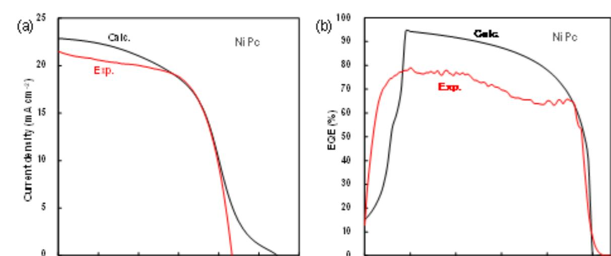
(a) Calculated J-V characteristics and (b) EQE of the perovskite solar cell using NiPc
