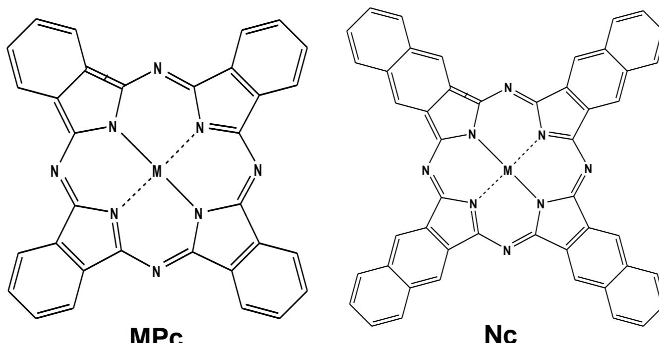
Molecular structure of MPc and Nc
