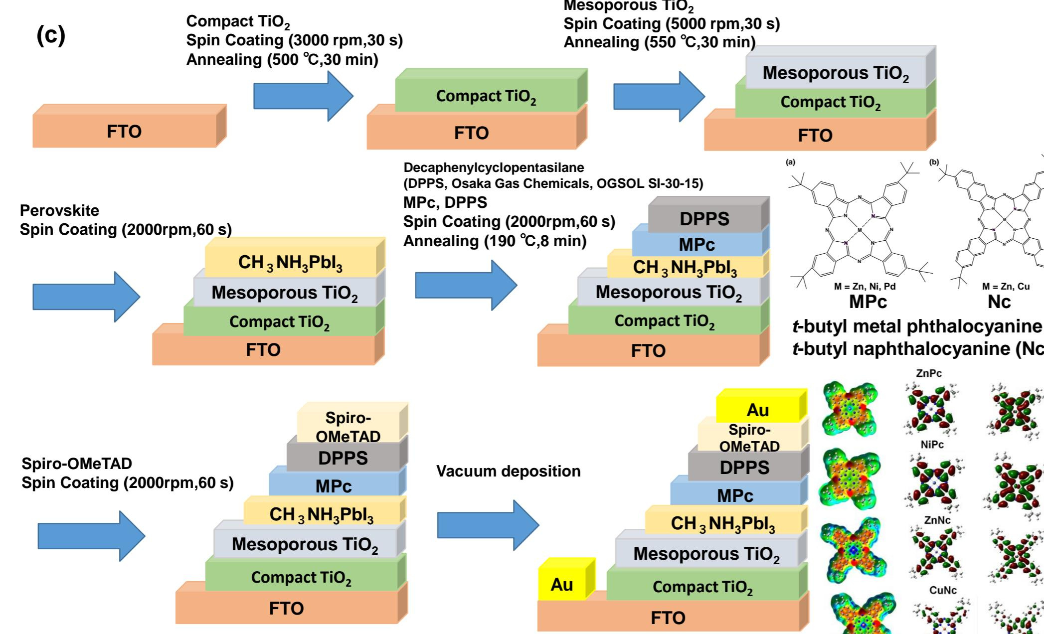
Fabrication of MAPbI<sub>3</sub> perovskite solar cell using MPc and Nc
