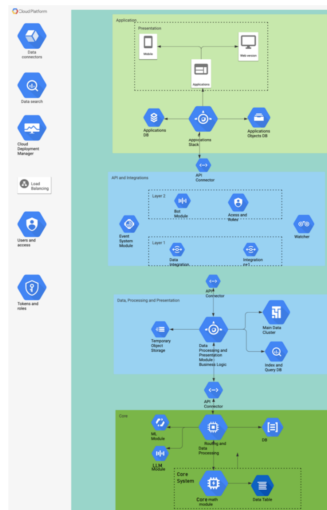
Figure 2. Three-layered Smart City cloud platform sub-services model
