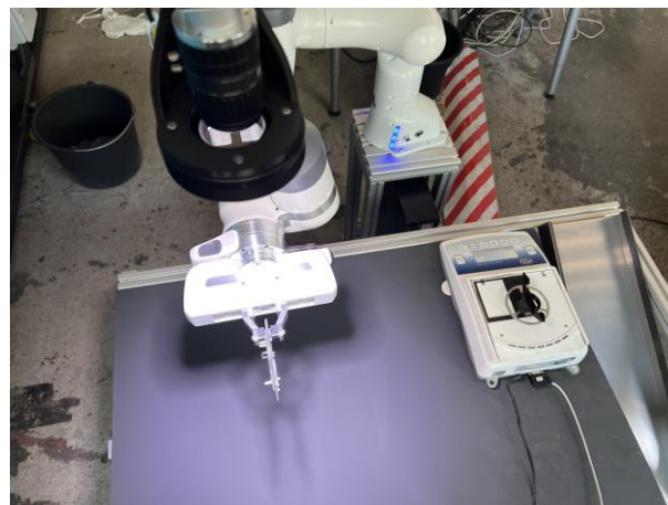
Figure 2. Overview of the used system setup consisting of the part handling robot, an industrial camera and a precision scale.
