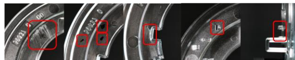
Figure 4. Examples of some of the artificially generated defects on the part surface marked in red. From left to right: scratches, dots, crack, missing structure 1, missing structure 2.
