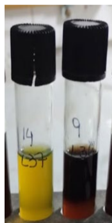
Fraser broth supplemented with ferric ammonium citrate showing negative and positive aesculin hydrolysis reaction, respectively.
