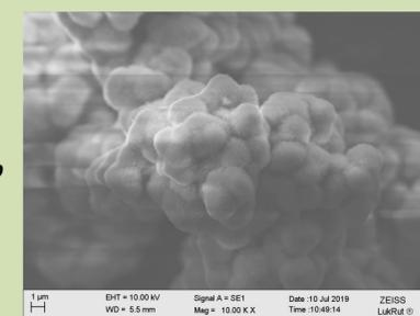
SEM images of FeOOH (a) and Nickel hydroxycarbonate (b)
