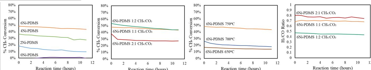
All reactions in this study are run with total flow of 60 ccpm, with results measured by gas chromatography. Parameters are 750°C, 1:1:1 CH<sub>4</sub>:CO<sub>2</sub>:N<sub>2</sub> unless otherwise stated
