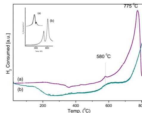
Figure 3: TPR diagram between ambient T and 820 °C for the phases: (a) MnMo<sub>9</sub> and (b) MnMo<sub>9</sub>/Diat.
