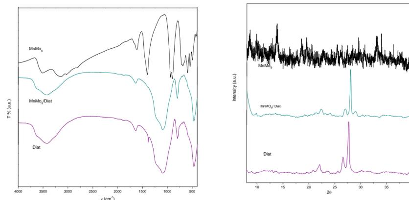
Figure 2: A) Comparative FTIR spectrum of MnMo<sub>9</sub>, diatomaceous earth and MnMo<sub>9</sub> supported on diatomaceous earth and B) DRX comparative
