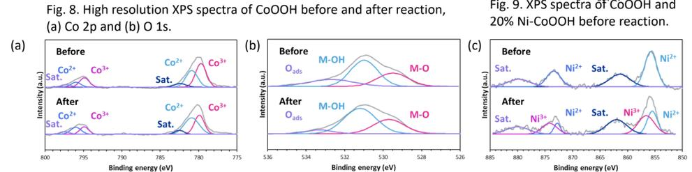
Fig. 10. High resolution XPS spectra of 20% Ni-CoOOH before and after reaction, (a) Co 2p, (b) O 1s and (c) Ni 2p.
