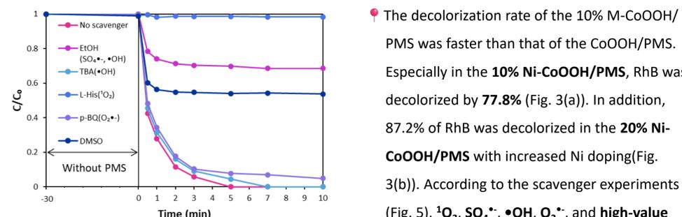
The decolorization rate of the 10% M-CoOOH/PMS was faster than that of the CoOOH/PMS. Especially in the **10% Ni-CoOOH/PMS**, RhB was decolorized by **77.8%** (Fig. 3(a)). In addition, 87.2% of RhB was decolorized in the **20% Ni-CoOOH/PMS** with increased Ni doping (Fig. 3(b)). According to the scavenger experiments (Fig. 5), <sup>1</sup>O<sub>2</sub>, SO<sub>4</sub><sup>•-</sup>, •OH, O<sub>2</sub><sup>•-</sup>, and **high-value metals** are thought to be involved in RhB decolorization.
