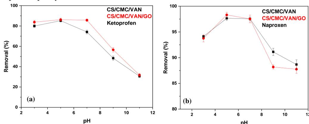
Fig 5. Effect of pH on the adsorption of (a) ketoprofen and (b) naproxen
