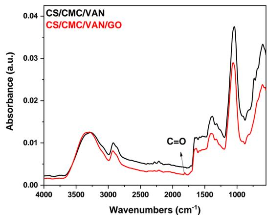
Fig 3. FTIR spectrum of CS/CMC/VAN and CS/CMC/VAN/GO
