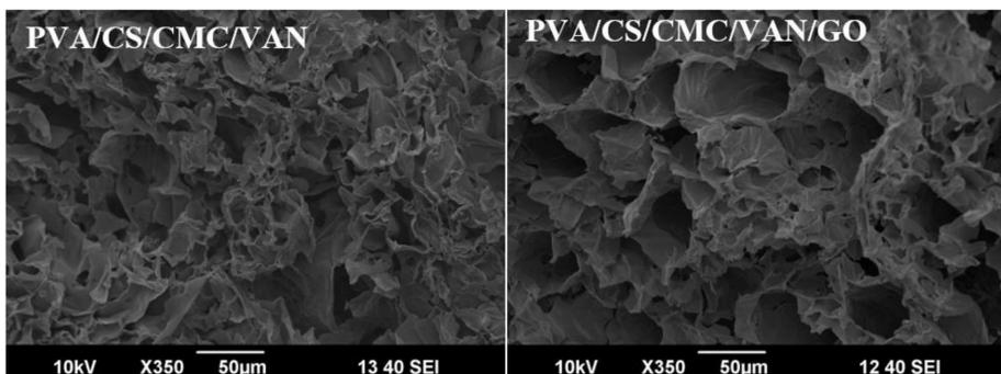
Fig 4. SEM images of CS/CMC/VAN and CS/CMC/VAN/GO
