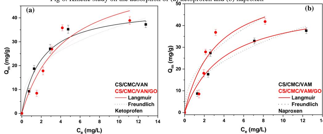
Fig 7. Isotherm study on the adsorption of (a) ketoprofen and (b) naproxen
