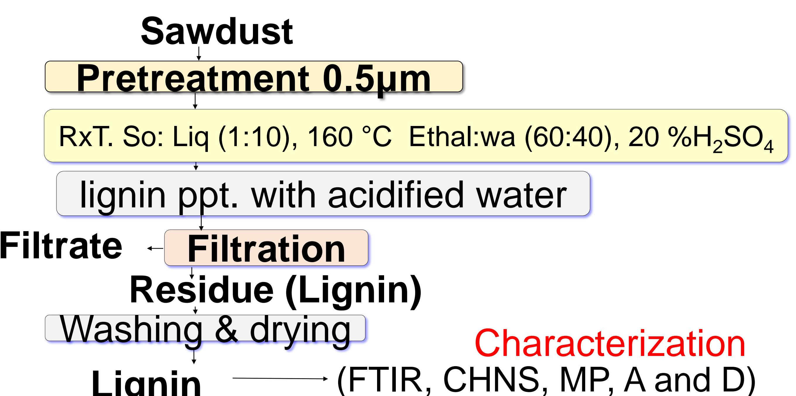
Figure 4: Experimental Procedure for Lignin Extraction
