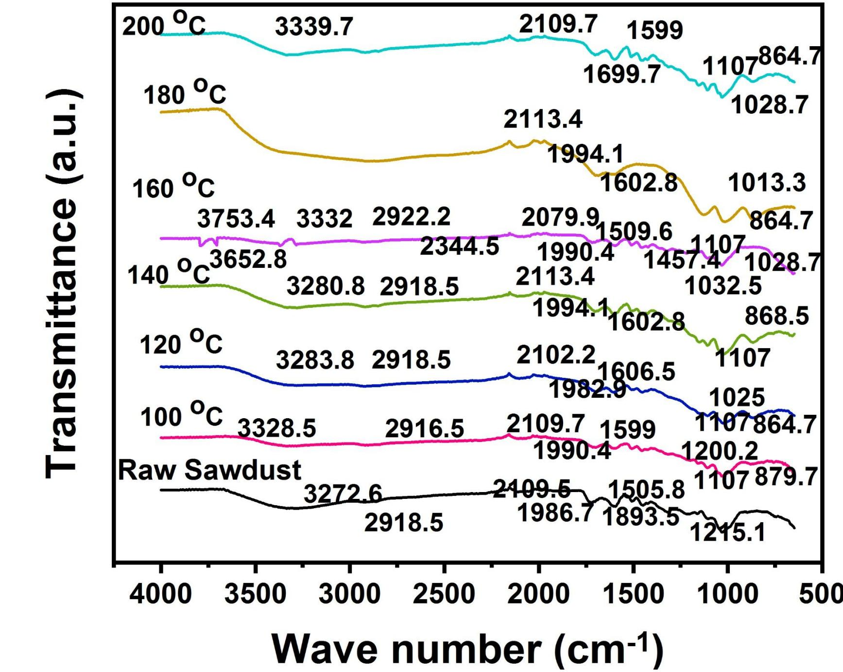
Figure 5: FTIR Analysis of Lignin from sawdust at 100, 120, 140, 160, 180 and 200 °C
