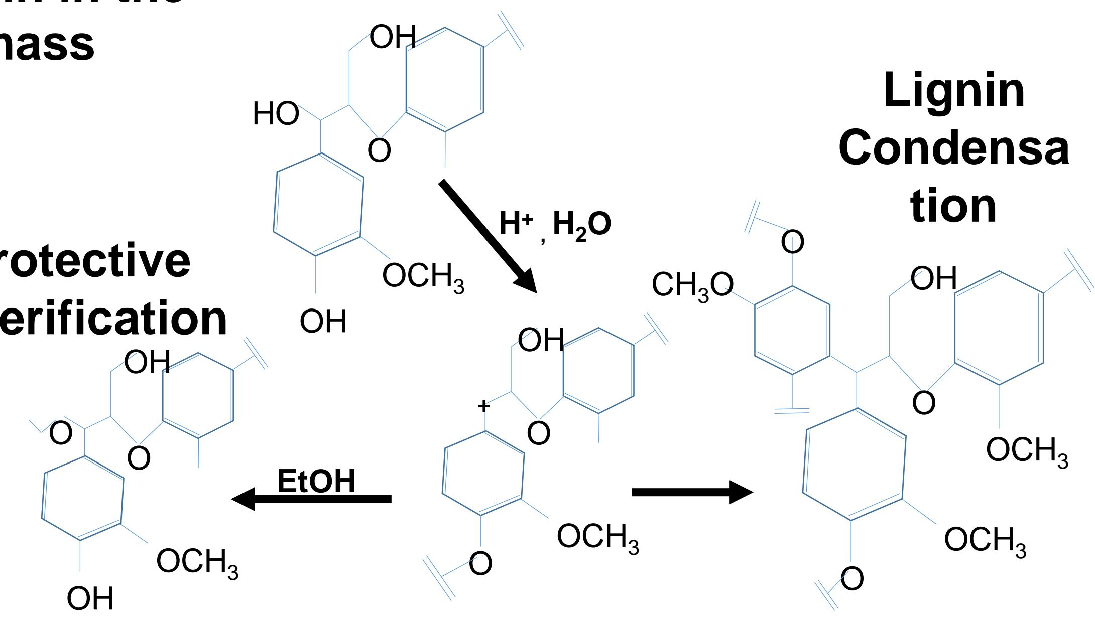
Figure 3: Lignin Extraction Mechanism in Organosolv Process (Du et al., 2021).
