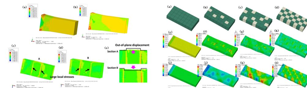
Fig. 4 Simulation results with different neighboring grain orientations and texture contents
