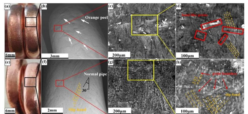
Fig. 1 Visual observation and SEM observations with (a)-(d) and without (e)-(h) orange peel tubes
