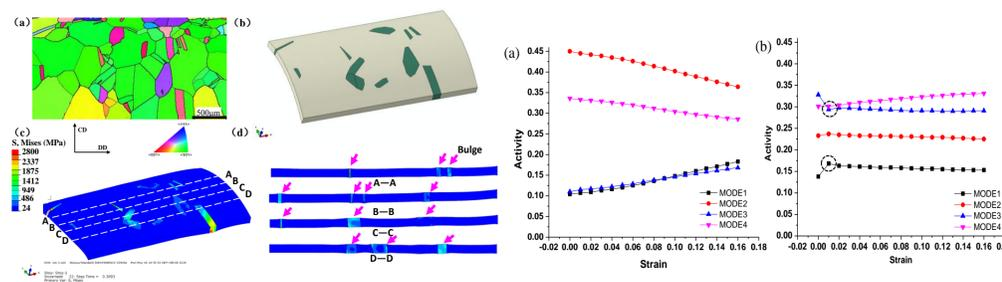
Fig. 5 RVE model and simulation results of surface morphology of orange peel tubes
