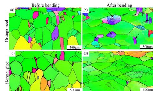
Fig. 2 Orientation distribution of tubes with and without orange peel defects before and after bending
