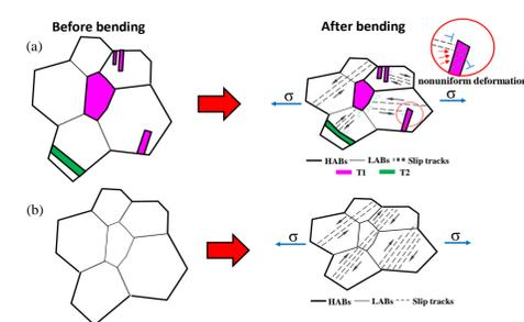
Fig. 3 Schematic diagram of orange peel formation mechanism on bent tube
