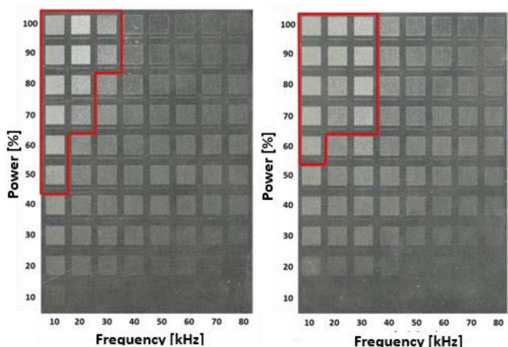
Figure 3: Aluminum AW-6082-T6 marked at 1 m/s (left) and 2 m/s (right).
