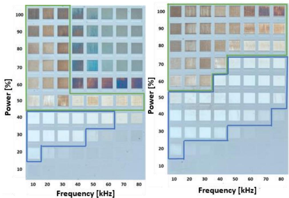
Figure 2: Stainless steel 304 2B marked at 1 m/s (left) and 2 m/s (right).
