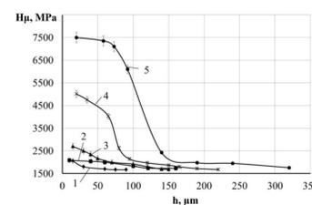
Figure 4 - Distribution of microhardness (H<sub>μ</sub> in the aluminised coating (h) on steel C20 during ESA with discharge energy: 1 – 0.52 J, 2 – 1.30 J, 3 – 2.6 J, 4 – 4.6 J, 5 – 6.8 J
