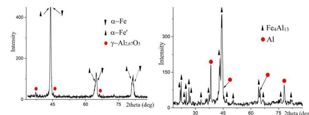
Figure 5 – Diffractograms of coatings on steel 20 after ESA alitisation at discharge energies: a – 0.52 J, b – 1.30 J
