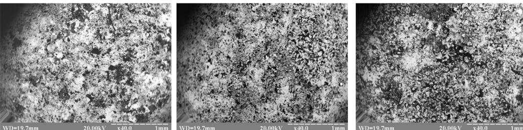
Figure 2 – Aluminised coating morphology on C20 steel after ESA at discharge energies: a - 0.52 J, b - 1.30 J, c - 2.6 J
