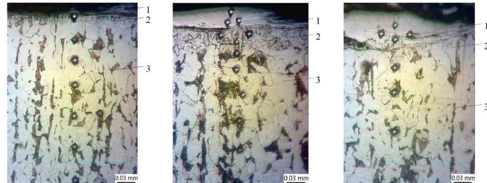
Figure 3 - Structure of the alitised coating (optical microscopy) on steel C20 after ESA at the discharge energy: a – 0.52 J, b – 1.30 J, c – 2.6 J.
