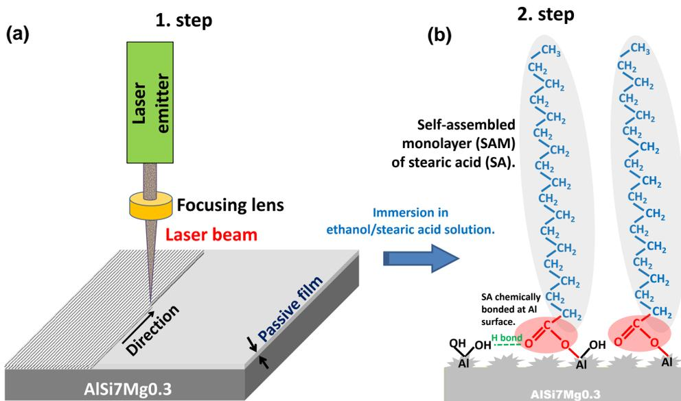
**Figure 1.** The scheme presents the two-step process to create a (super)hydrophobic aluminium surface. The first step consists of laser structuring of the aluminium surface (a) and (b), followed by grafting with stearic acid (SA).
