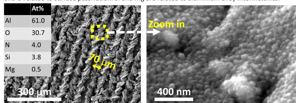
**Figure 2.** Secondary electron SEM images of laser-structured surfaces prepared using laser scanning line spacing modified with stearic acid. EDS spectrum and surface composition are given in atomic percentages (at. %); carbon is excluded.
