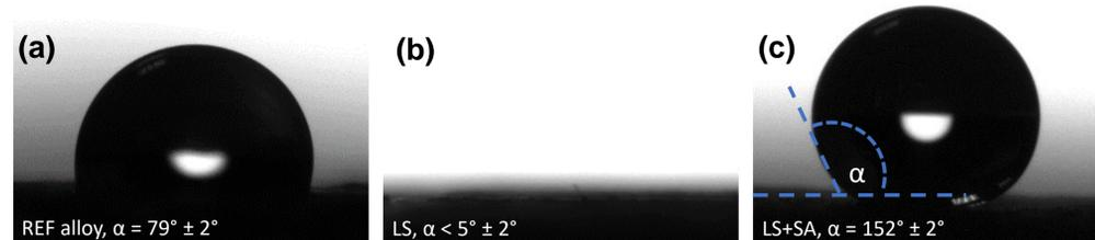
**Figure 3.** Wettability of the (a) REF surface, (b) laser-structured alloy and (c) grafted with stearic acid.
