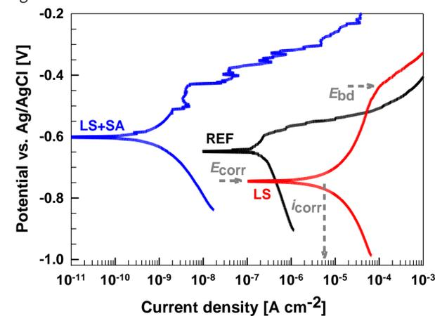
**Figure 4.** Potentiodynamic polarisation measurements after one hour of immersion in 0.1 M NaCl solution for laser-structured AlSi7Mg0.3 samples prepared without and with modification of stearic acid.
