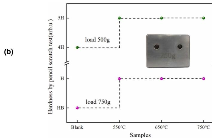
(a) Preparation of cement-based inorganic cementitious coating, (b) Pencil hardness test on coatings. (Wang, Pei et al. 2025).
