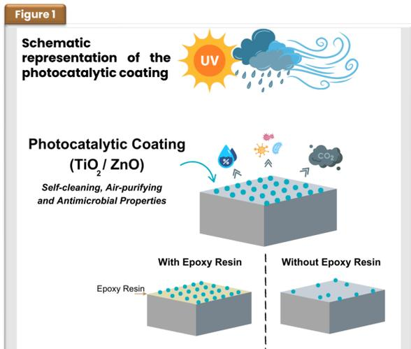
This research aims to develop self-cleaning cement-based panels functionalized with TiO<sub>2</sub> and TiO<sub>2</sub>/ZnO, and to evaluate the impact of epoxy resin on their photocatalytic activity and aesthetic properties.
