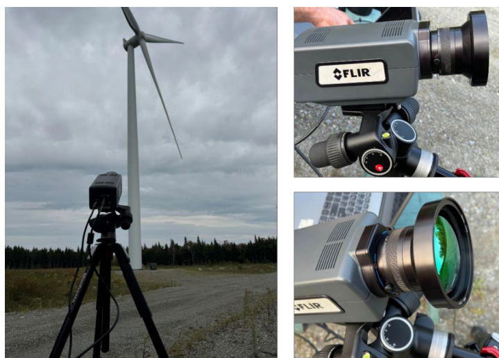
Figure 4. Infrared Camera Setup with 100 mm Lens for Blade Inspection
