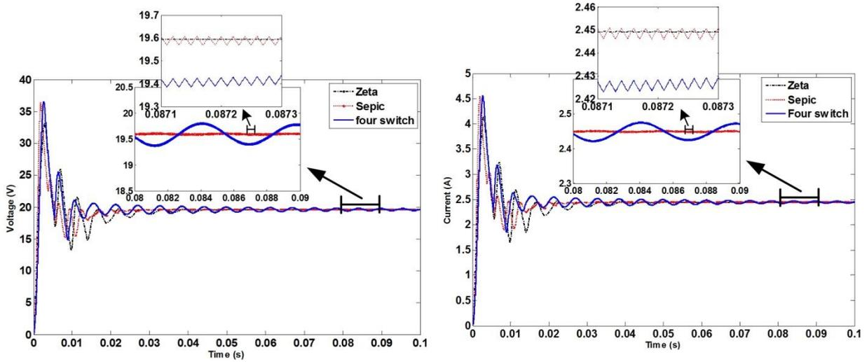
Figure 11. Voltage and current outputs from PV emulator for different buck-boost converter topologies loaded with  $8\ \Omega$  resistor.
