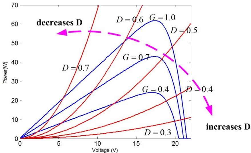
Figure 13. Power characteristics of the PV system.
