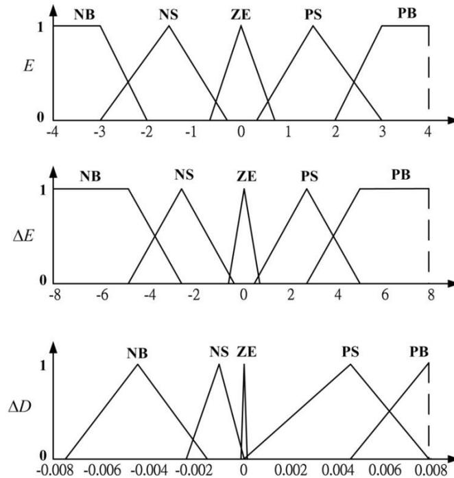
Figure 15. Membership functions for the input and output variables.
