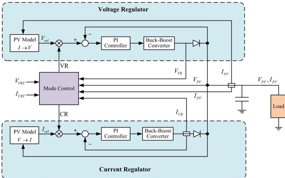
Figure 6. Block diagram of the dual-mode PV emulation system
