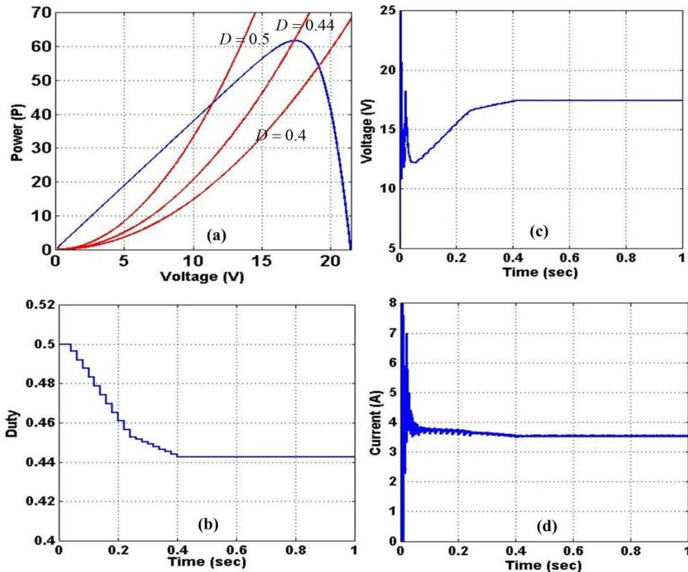
Figure 17. Circuit simulation results with  $3\ \Omega$  load. (a). Power characteristics. (b). Duty ratio command. (c). Output voltage from PV emulator. (d). Output current from PV emulator.
