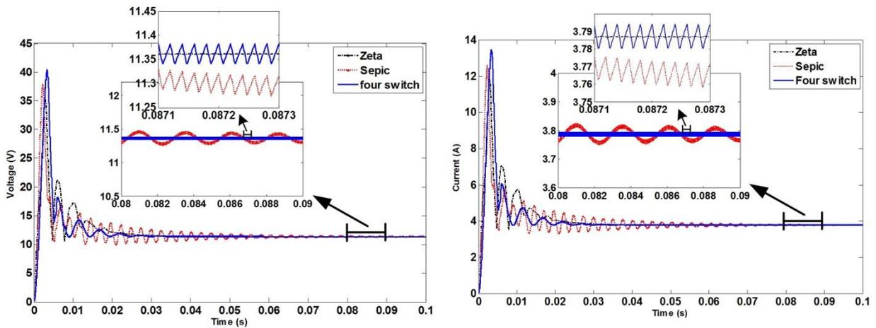
Figure 9. Voltage and current outputs from PV emulator for different buck-boost converter topologies loaded with 3 Ω resistor.
