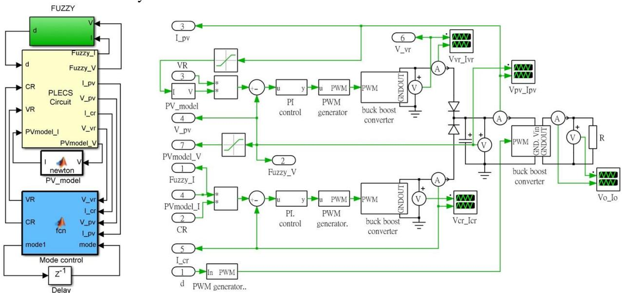
Figure 16. Circuit simulation model for buck-boost converter based MPPT system with its PLECS circuit.
