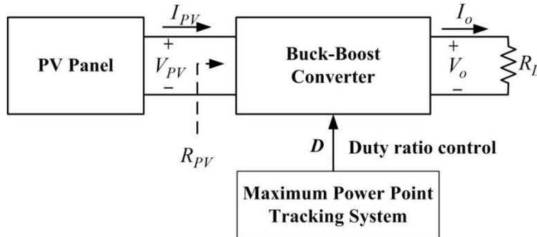
Figure 12. PV system with buck-boost converter incorporated.
