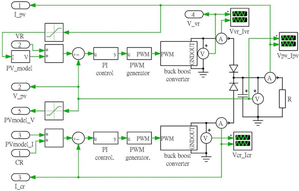
Figure 8. PLECS circuit simulation model for PV emulation with resistive load
