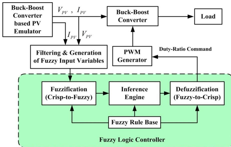
Figure 14. Fuzzy logic controller for the MPPT design.
