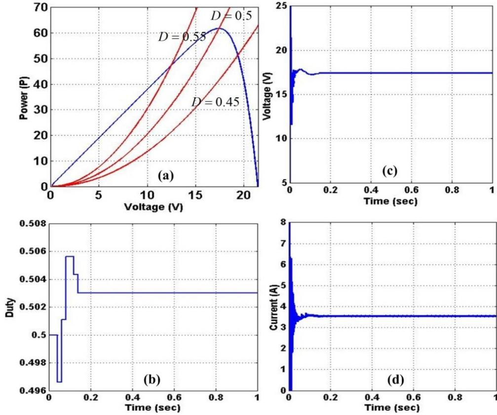
Figure 18. Circuit simulation results with  $4.9\Omega$  load. (a). Power characteristics. (b). Duty ratio command. (c). Output voltage from PV emulator. (d). Output current from PV emulator.
