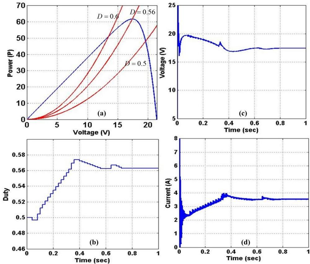
Figure 19. Circuit simulation results with  $8\Omega$  load. (a). Power characteristics. (b). Duty ratio command. (c). Output voltage from PV emulator. (d). Output current from PV emulator.
