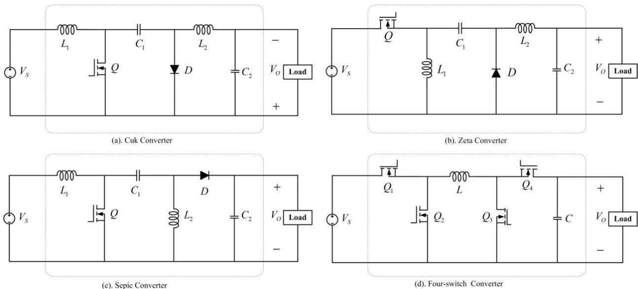
Figure 2. Buck-Boost Converters. (a). Cuk converter, (b). Zeta Converter, (c). SEPIC Converter, (d). Four-switch type converter.
