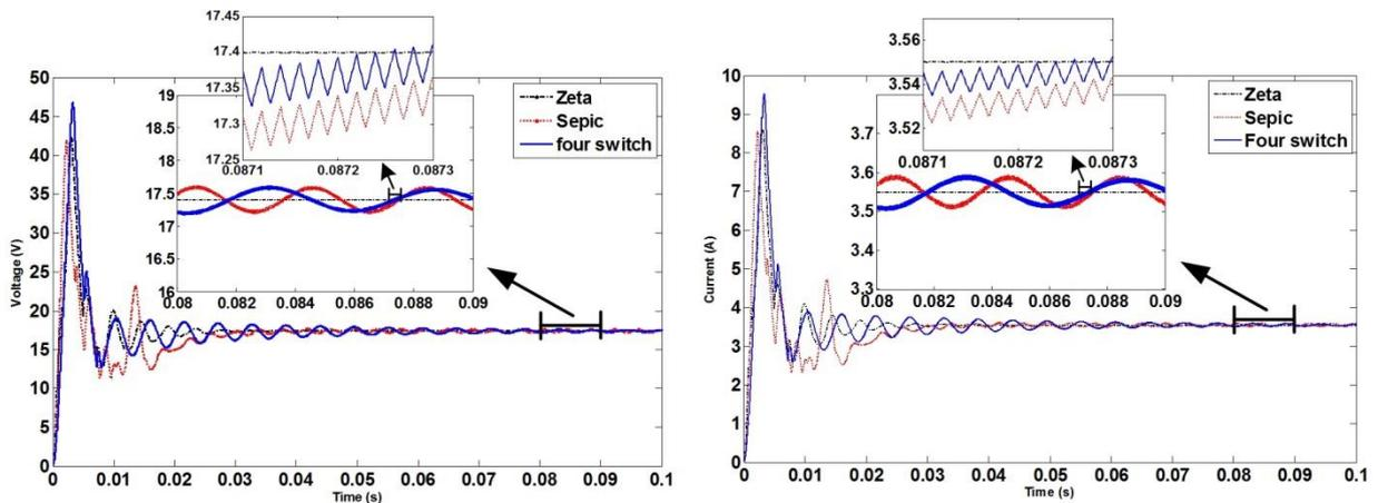
Figure 10. Voltage and current outputs from PV emulator for different buck-boost converter topologies loaded with 4.9 Ω resistor.
