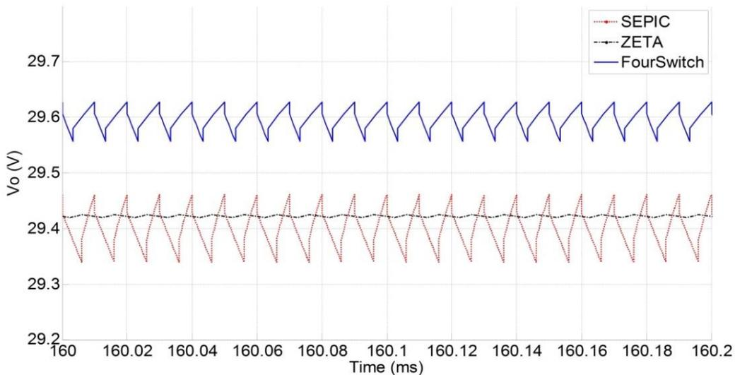
Figure 4. Comparison for steady-state responses
