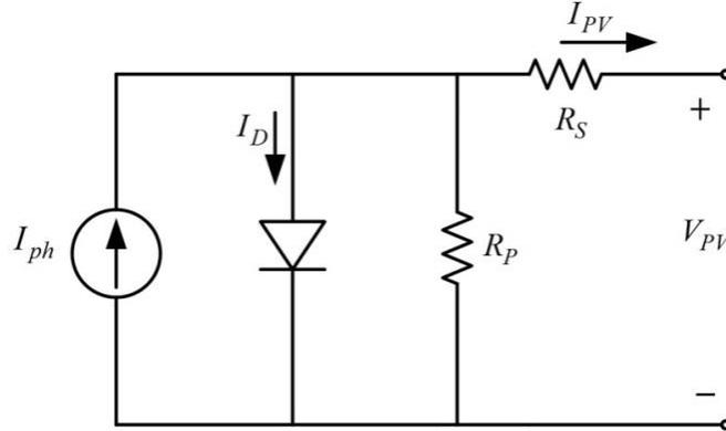
Figure 1. Single-diode equivalent circuit model
