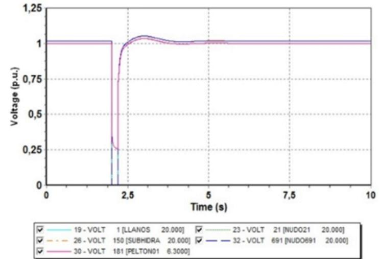
Voltage dips in isolated systems are very deep and their area of propagation is very wide-spread.
